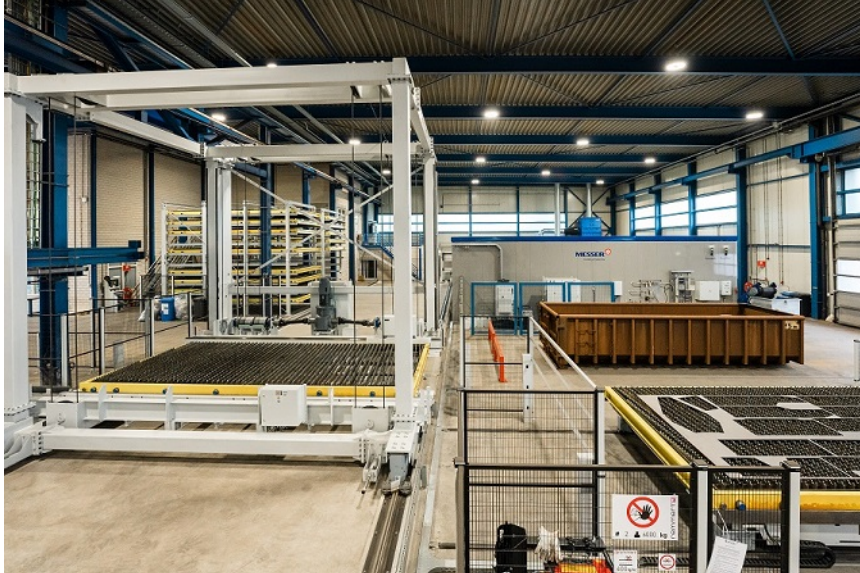
Photo 8: The software suite OmniFab connects the various software systems, cutting machines as well as the Remmert Material Handling System via various interfaces. © Messer Cutting Systems
