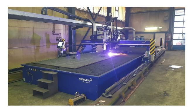
Caption 2: Equipped for complex cutting tasks: Thus, for example, internal contours can be cut with oxyfuel and outer contours with plasma in combination.
