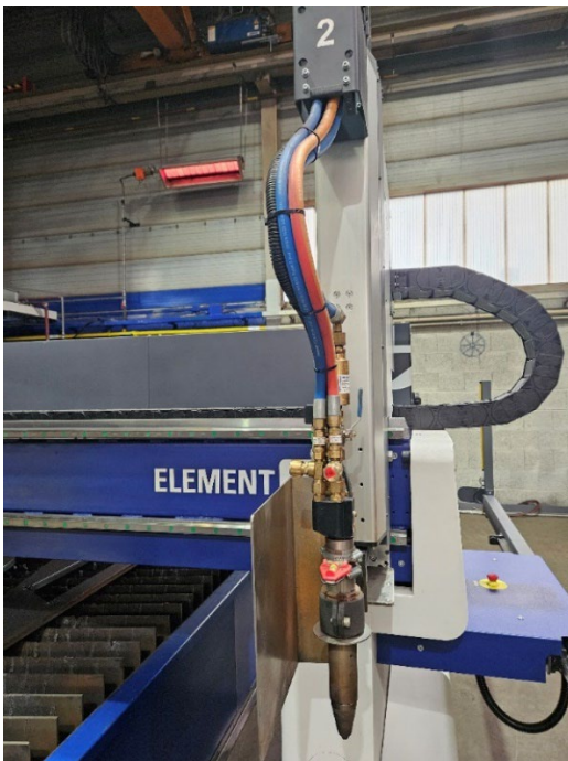
Image 2: Messer oxyfuel cutting torch ALFA: Improved material utilisation through optimal sensing and cutting, also along the edges.
