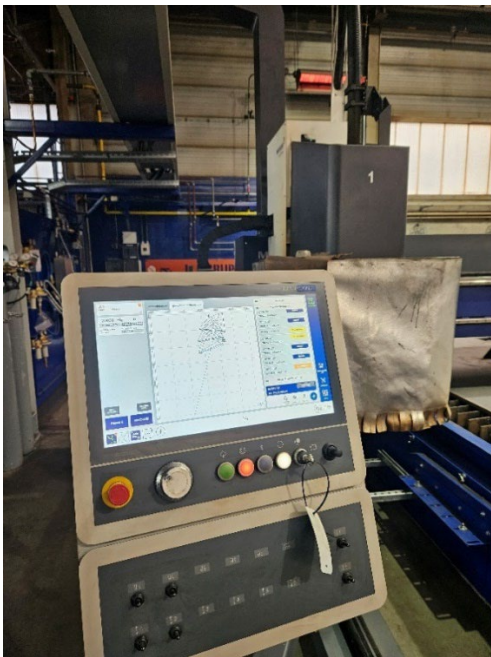
Image 3: Easy-to-use Global Connect control with nesting plan from the OmniWin CAD/CAM software.
