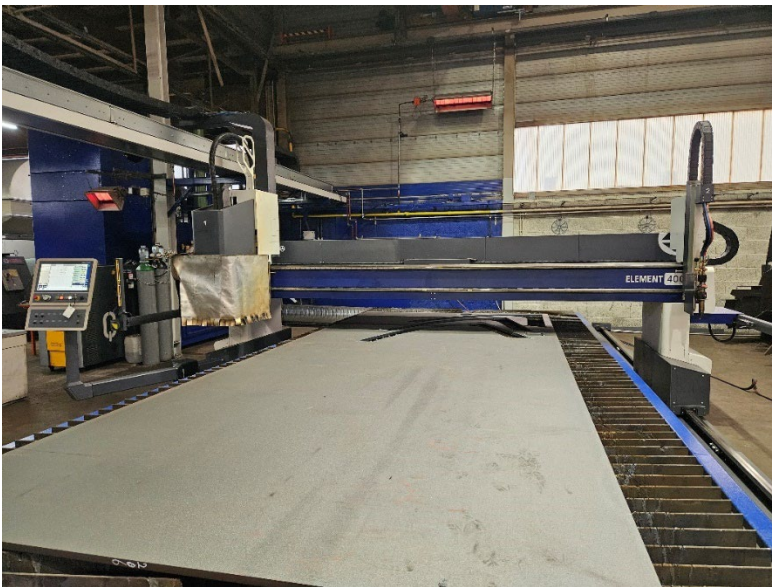
Image 1: The ELEMENT machine with plasma bevel unit Bevel-S and ALFA oxyfuel torch from Messer Cutting Systems.
