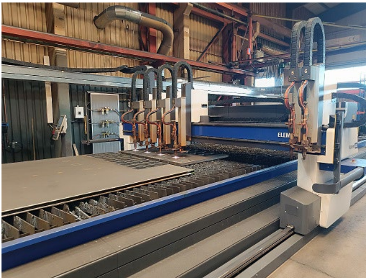
Caption 3: Four of the six oxyfuel machine torches ALFA in action on the ELEMENT, © Wagner Stahl
