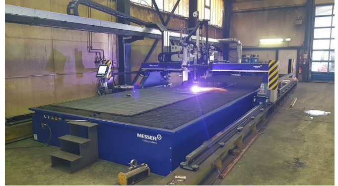
Caption 1: Equipped for complex cutting tasks: Thus, for example, internal contours can be cut with oxyfuel and outer contours with plasma in combination.
