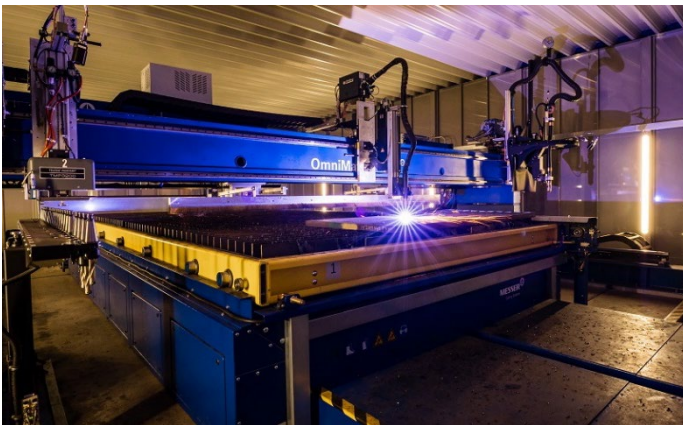
Caption: OmniMat® cutting machine equipped with the Skew Delta plasma bevel unit for weld preparation
