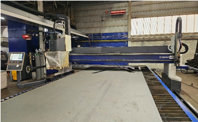
Caption: The ELEMENT machine with plasma bevel unit Bevel-S and ALFA oxyfuel torch from Messer Cutting Systems.
